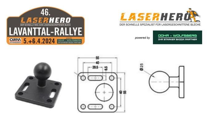
The device will be attached to a 1 inch ball head as shown in the picture above. This ball mount must be attached to the vehicle with tight screws at a location as described above. The diameter of the screw holes is 6.5mm and the distance between the holes is 40mm. When mounting on the dashboard, a support plate must be attached to the back to prevent the screws from breaking through the plate in the event of an accident to prevent the holder from flying around freely in the vehicle.
